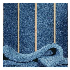
The cotton is then treated with a borate solution, a low toxicity biodegradable flame-retardant. This solution is free from VOCs and formaldehyde. This type of insulation was developed in the 1990s from the enormous amount of scrap denim sourced from clothing manufacturers. Some upsides to using this kind of insulation are that it doesn't contain formaldehyde, doesn't cause respiratory problems, is biodegradable, and is a natural
