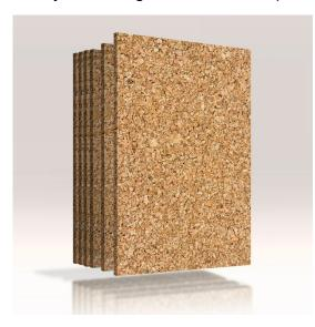
The only materials involved are the bark itself and steam from a high temperature boiler. The process involves steam-heating cork granules, which are then pressed into a board, causing the cork to expand. This activates a natural binder known as suberin, which fuses the granules. No other binders or chemicals are used in the process. It's renewable, recyclable, and biodegradable. Thermacork utilizes cork that
